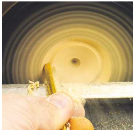
▲ Pic.23 Hold the tool firm and start the hallowing. Using your left thumb as a back stop will help when making the incision. Move the tool round in an arc
